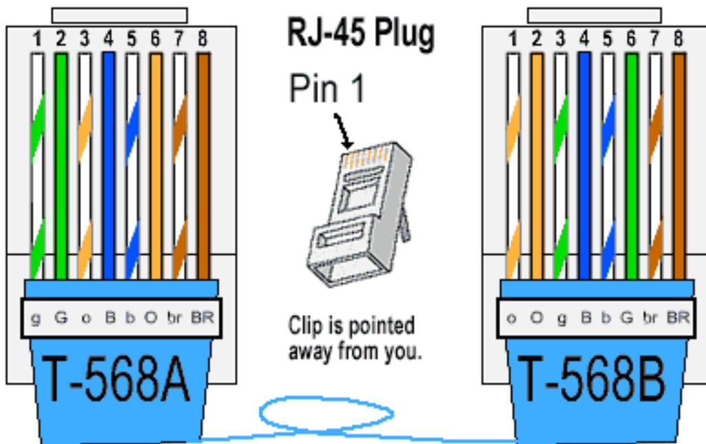
A good way of remembering how to wire a Crossover Ethernet cable is to wire one end using the T-568A standard and the other end using the T-568B standard. Another way of remembering the
