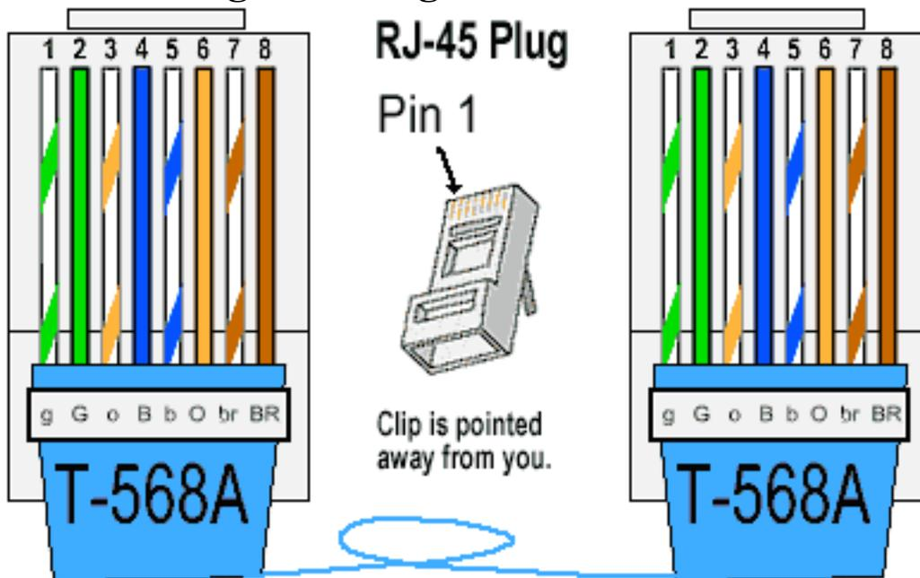
The T-568A standard is supposed to be used in new network installations. Most off-the-shelf Ethernet cables are still of the T-568B standard; however, it makes absolutely no functional difference in which you choose.
